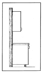
Cabinets can be mounted with ease and accuracy. They can be placed anywhere along the horizontal track and can be changed in seconds when needed.
