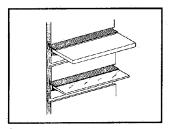
Since the shelves are supported over their entire length, they do not sag unevenly under load. Also where RAKKS brackets are used metal or plastic inserts are not necessary.
